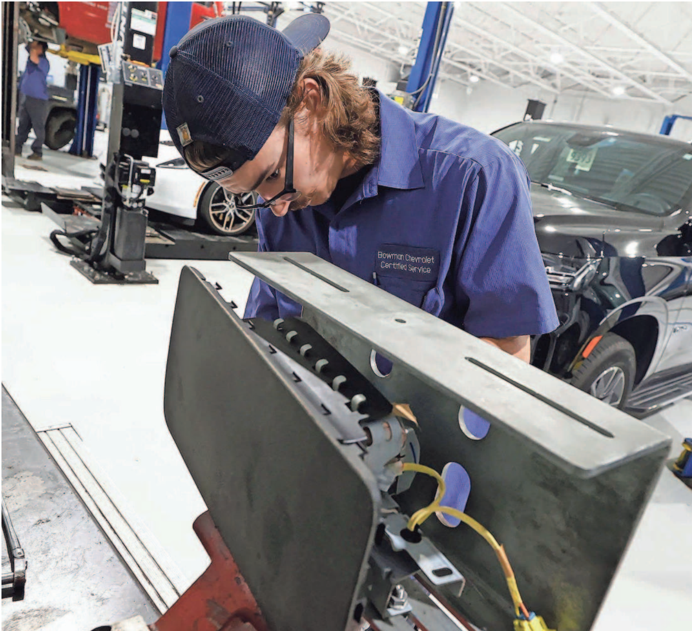
Bowman Chevrolet service technician Anthony Carbone, 22, removes a recalled Takata front passenger airbag from a Chevrolet Silverado before replacing it with a new one at the dealership in Clarkston, Mich. ERIC SEALS/USA TODAY NETWORK
