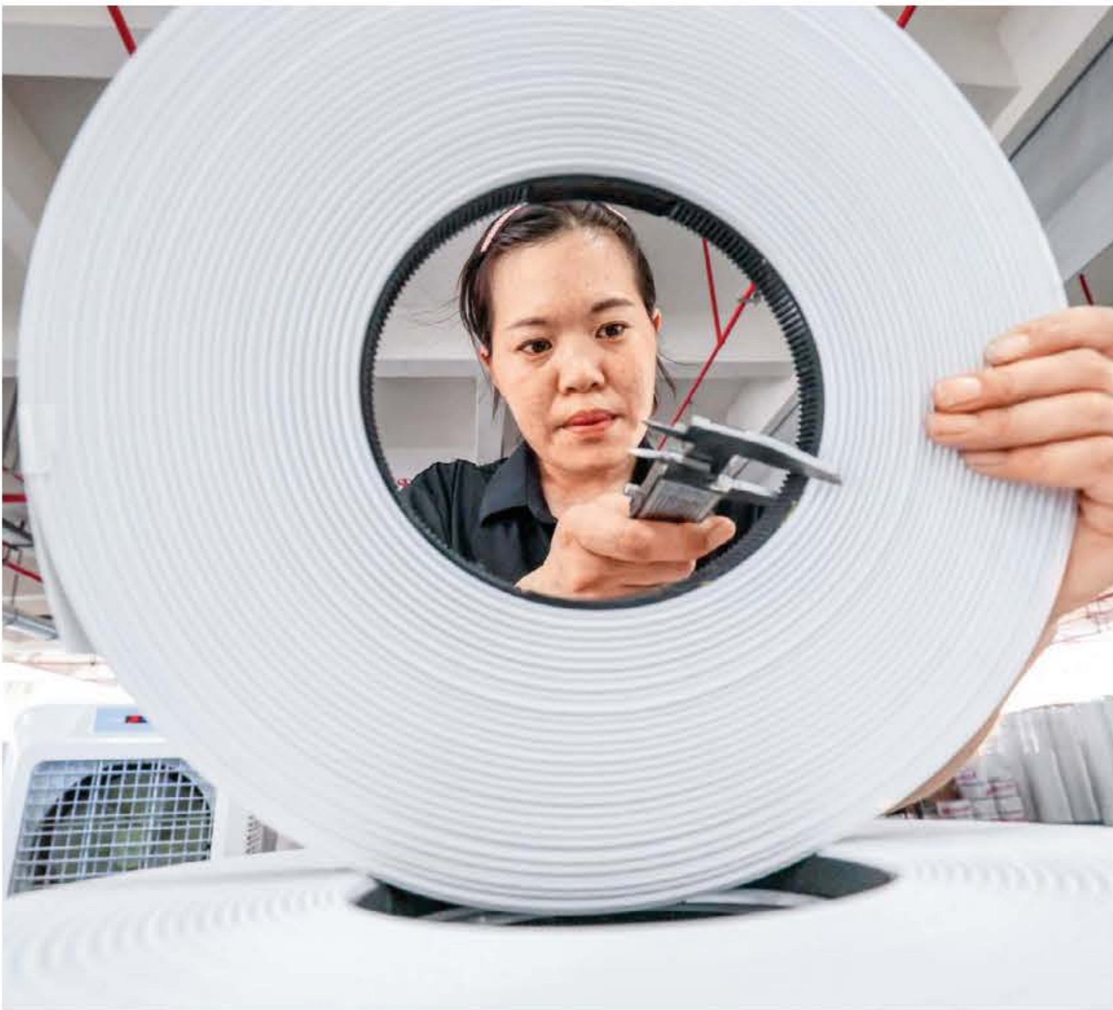
A worker produces an order for edge banding for export to Europe at a decorative materials workshop in Huzhou city, Zhejiang province. Edge banding is used in carpentry to cover the exposed sides of materials such as plywood or particle board,
