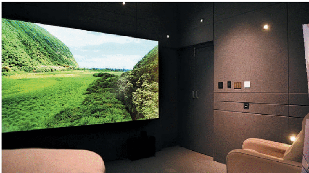
A 4K acoustically-perforated screen for a minimalistic approach where speakers are behind the screen with lighting fixtures made of wood to complement the acoustical treatment in the room
