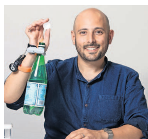
Kaya Burgess opens a bottle with one hand as he tests a robotic third thumb
