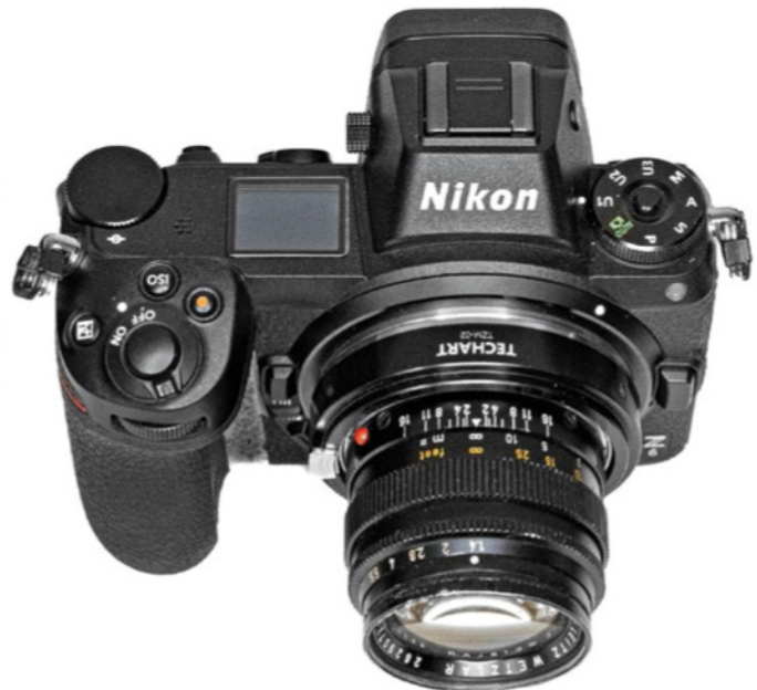
Picture 6: A Nikon Z6 camera with an AF-capable Techart TZM-02 Adapter along with the same lens as shown in Picture 5.
