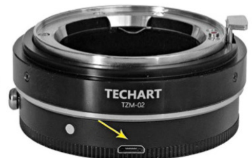
Picture 4: Two views of the Techchart TZM-02 MF to AF adapter from both sides. The contacts of the adapter (red arrow) mate with the camera to send / receive data and commands. The other side interfaces to an MF lens and hence needs no contacts. AF technology is continuously evolving and the USB port (yellow arrow) provided on the specially designed cap can be used to update the firmware of the adapter.
