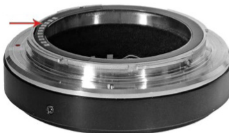
Picture 4: Two views of the Techchart TZM-02 MF to AF adapter from both sides. The contacts of the adapter (red arrow) mate with the camera to send / receive data and commands. The other side interfaces to an MF lens and hence needs no contacts. AF technology is continuously evolving and the USB port (yellow arrow) provided on the specially designed cap can be used to update the firmware of the adapter.
