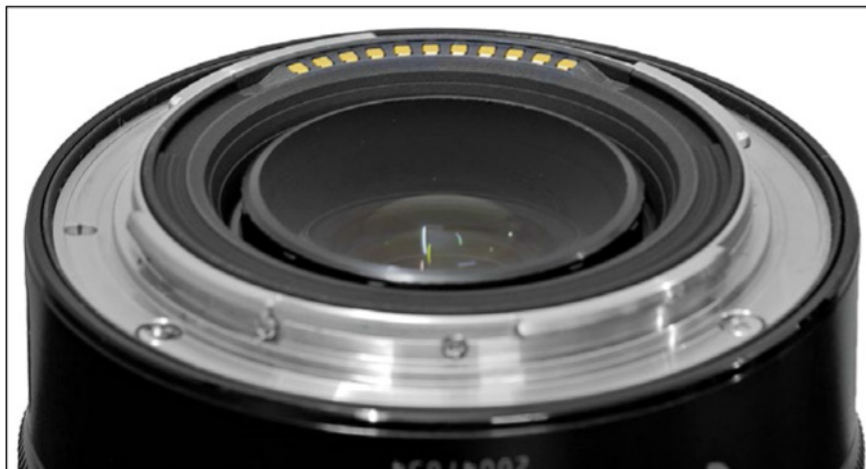
Picture 1: Electronic contacts of the lens. These receive the signals from the camera body and drive the focusing mechanism.
