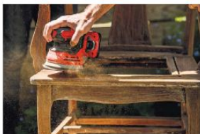
Finish the job by sanding, gradually moving from a coarser to a finer grit of sandpaper.
