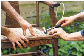
To add a cane seat, soak the material in water before driving it into the groove running around the chair. Add wood glue and a reed spline to lock the cane in place.
