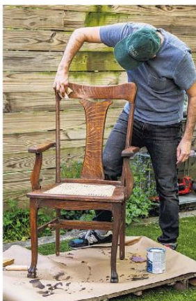
Complete the job with clear polyurethane. To avoid brushstrokes, it's best to use a fresh paintbrush or rag.
