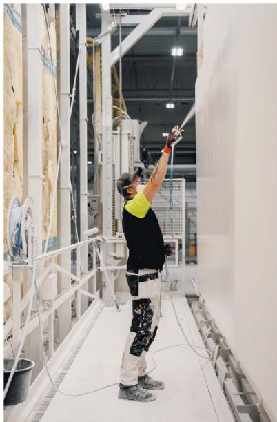
From top: a door frame being installed at the Lindbäcks modular construction factory in Sweden; a roof being installed; and a roof section being painted vertically. Housing modules simultaneously assemble lines cut down on delays. At Lindbäcks, one unit of volumetric housing is created every half an hour.
