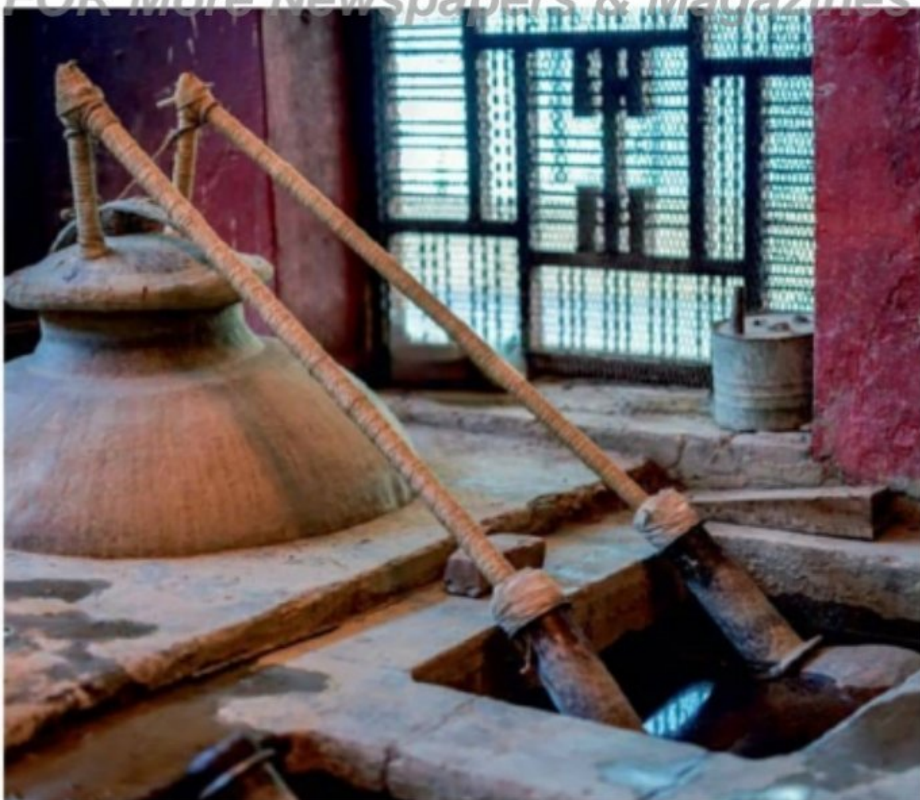
Steam distillation: Over 40 kgs of rose petals give just three grams rose oil
