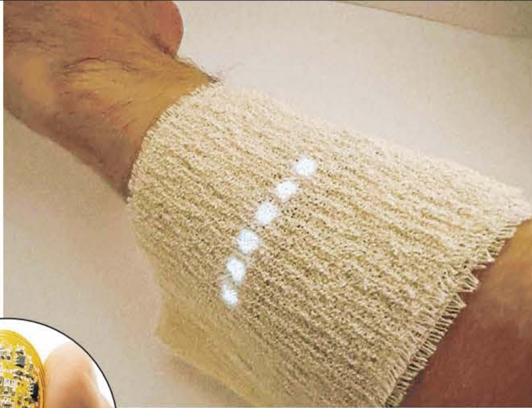
A smart bandage uses tiny LED lights to emit ultraviolet-C light. Left, flexible circuitry for a smart bandage.
