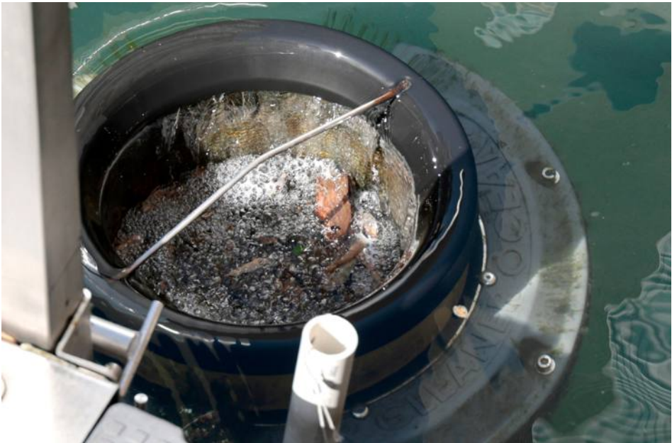
The Trash Trap collects litter in the Chicago River on Wednesday. It works by drawing in water and debris from the surface using a submersible pump, trapping litter inside a catch bin and pumping the water back out.
