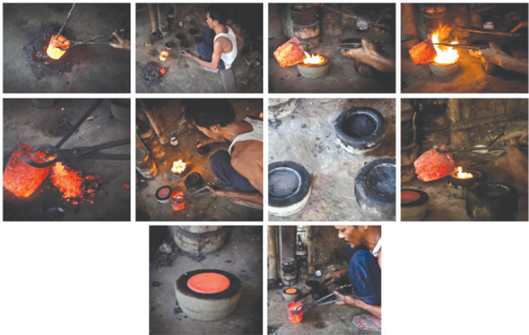
Figure 1: The stages involved in the solidification of the molten metal.
